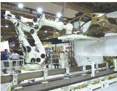
In December 2015, Kawasaki released the MG10HL, an ultra-high payload robot with maximum payload capacity of 1 ton. It demonstrated its capabilities by lifting a car body at the International Robot Exhibition 2015.
