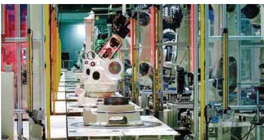
Inside the KPM (Suzhou) factory. Human workers perform tasks they are good at such as temporarily tightening bolts, while robots are assigned to tasks they excel at such as precision transporting and assembly.
