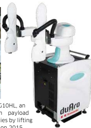
duAro, a dual-arm SCARA robot suitable for multi-product and small-lot productions collaborating with people safely and securely.
