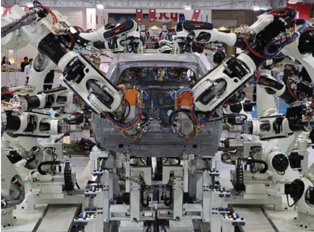
Large general-purpose B series robots launched in September 2011. The spot welding demonstration on an automobile body assembly line was exhibited at the International Robot Exhibition 2013.
