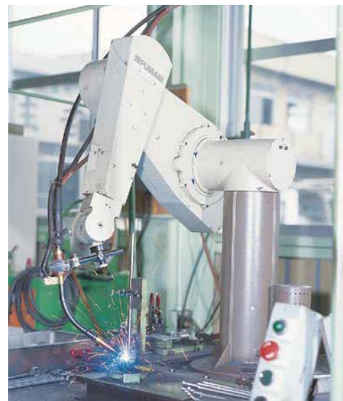
The electric-driven small articulated robot, PUMA, welding.
