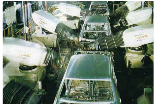
The Kawasaki-Unimate 2000 in operation at a car factory.
